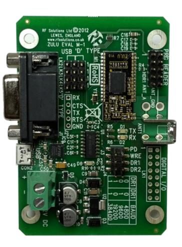
The ZULU EVAL Broad provides a ready made platform which can be used to demonstrate the capabilities of ZULU modem modules providing ready made RS232 and USB modem solutions.
