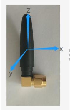
H plane: the tangent of XY E1 plane: the tangent of XZ E2 plane: the tangent of YZ
