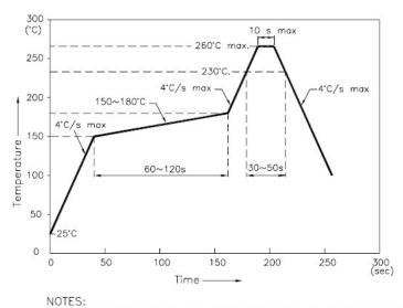
Reflow Soldering Profile For Lead-free SMT Process.
