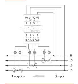
The correct type of measuring transformer must be set in the Fox application (for the Energy 3 module): **Module** settings → Measuring transformer.
