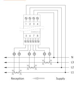
The correct type of measuring transformer must be set in the Fox application (for the Energy 3 module): Module settings  $\rightarrow$  Measuring transformer.
