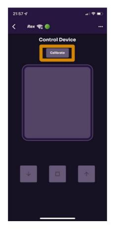
Then follow the on-screen instructions. The first step is to put the shutter into the top position. Press the **Start calibration** button on screen to start moving the shutter up.
