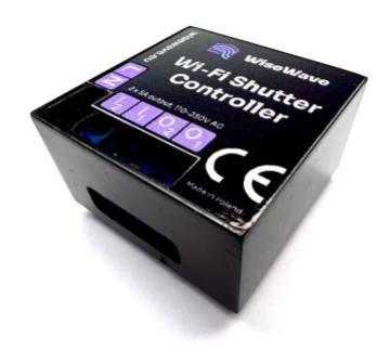
Wi-Fi Shutter Controller is – as the name suggests – an intelligent shutter controller. You can control it using WiseWave app as well as via inputs marked as II i I2, which allow you to expand or roll up the shutter.
