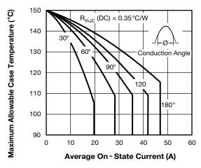
Fig. 1 - Current Rating Characteristics
