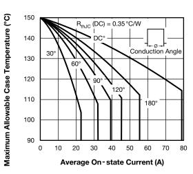
Fig. 2 - Current Rating Characteristics
