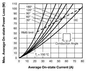
Fig. 4 - On-State Power Loss Characteristics
