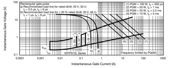
Fig. 8 - Gate Characteristics
