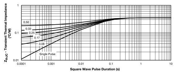
Fig. 9 - Thermal Impedance Z<sub>thJC</sub> Characteristics
