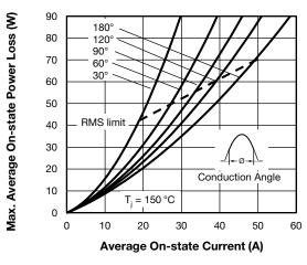
Fig. 3 - On-State Power Loss Characteristics
