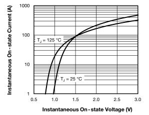
Fig. 7 - On-State Voltage Drop Characteristics
