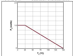
**FIGURE 2-5:** Power Dissipation vs. Case Temperature.
