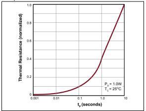
**FIGURE 2-6:** Thermal Response Characteristics.
