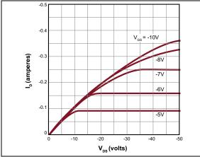
FIGURE 2-1: Output Characteristics.
