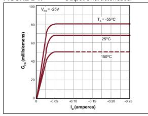
**FIGURE 2-2:** Transconductance vs. Drain Current.
