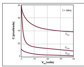
**FIGURE 2-9:** Capacitance vs. Drain-to-Source Voltage.
