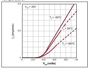
FIGURE 2-8: Transfer Characteristics.
