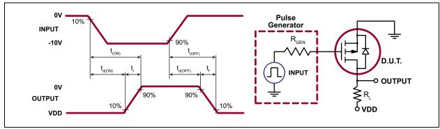
FIGURE 4-1: Switching Waveforms and Test Circuit.
