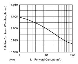
Fig. 3 - Relative Dominant Wavelength vs. Forward Current
