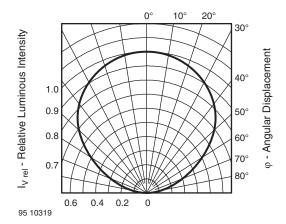
Fig. 2 - Relative Luminous Intensity vs. Angular Displacement
