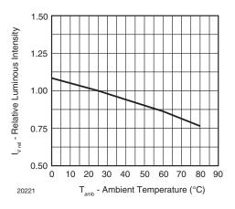
Fig. 6 - Relative Luminous Intensity vs. Ambient Temperature
