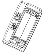
1. Open the battery cover. Then, set the slide switch to **Setup**.
