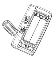
2. Use a flat-blade screwdriver to push the button located in the hole for around three seconds.
