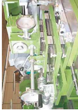
The adjustment of the pressing roller and the compensation of the imbalance of the grinding tools are implemented with drylin® T in place of recirculating ball bearing guides.
