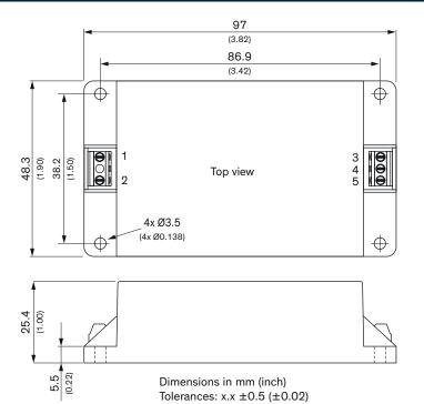
Mounting screw locked torque: 0.2 Nm (2 kgfcm)
