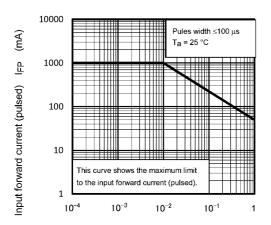
Duty cycle ratio D<sub>R</sub> Fig. 11.3 I<sub>FP</sub> - D<sub>R</sub>
