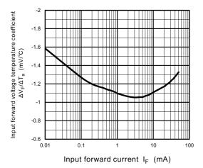
Fig. 11.5  $\Delta V_F/\Delta T_a - I_F$
