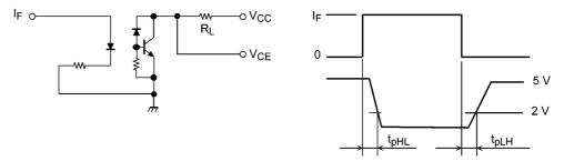
Fig. 10.1 Switching Time Test Circuit and Waveform
