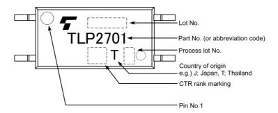
Note: A different marking is used for photocouplers that have been qualified according to option (D4) of EN 60747.
