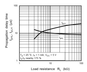
Fig. 11.14  $t_{pHL}$ ,  $t_{pLH}$  -  $R_L$
