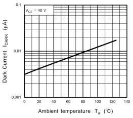
Fig. 11.9 I<sub>DARK</sub> - T<sub>a</sub>
