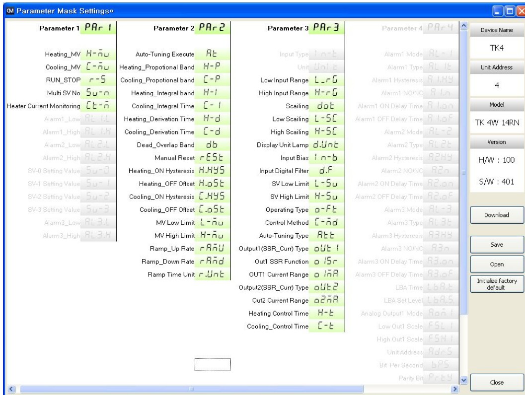
Example of masking alarm, SV setting parameters of parameter 1 group, input type, unit of parameter 3 group, and all of parameter 4 group.
