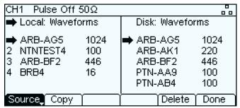
Waveforms and set-ups can be stored on a USB Flash drive as well as within the instrument
