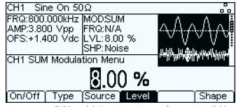
SUM modulation generates waveforms not available through conventional modulation schemes \*
