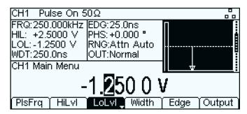
Output levels can be entered as high level and low level as an alternative to amplitude and offset
