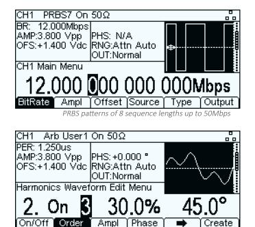
The harmonics generator enables waveforms to be constructed using up to 16 sine harmonics
