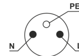
PE – safety contact | N – neutral contact | L-phase contact Fig. 1 The pin grid array of the power socket (PN-E-93201:1997)
