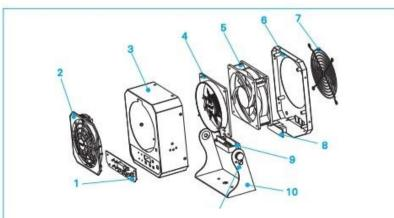
Control panel 2. Front air window 3. Front shell 4. Spray point component 5. Fan 6. Back cover 7. Metal rear air window 8. Power input board 9. Ion generator 10. Support 11. Angle fixed screw
