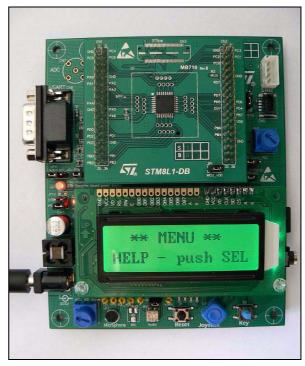
The full range of hardware features on the STM8L101-EVAL helps you to evaluate all peripherals (micro SD Card, USART, EEPROM, LCD, for example) and develop your own applications.
