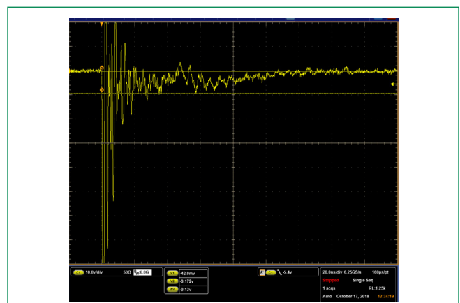
IEC 61000-4-2 -8 kV Contact ESD Clamping Voltage
