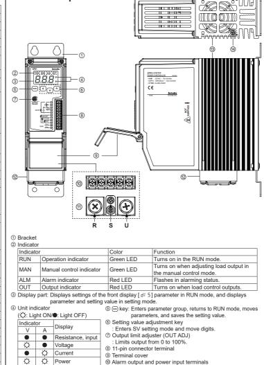
Cooling fan: For models with the rated load current of 70A/100A/150A, a cooling fan is attached
