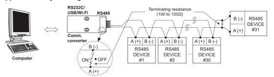
※It is recommended to use Autonics communication converter; SCM-WF48 (Wi-Fi to RS485·USB wireless communication converter, sold separately), SCM-US48I (USB to RS485 converter, sold separately), SCM-38I (RS232C to RS485 converter, sold separately). Please use twisted pair wire, which is suitable for RS485 communication, for SCM-WF48, SCM-US48I and SCM-38I.
