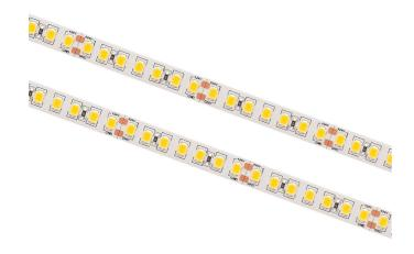
High quality LED strip for professional use with seven LEDs in one module to achieve luminous efficacy up to 140 lm/W. Two layers of PCB with 3oz copper paths characterized by a lower voltage drop and lower operating temperature. On a base using adhesive tape 3M 300 LSE. LEDs that meet requirements of LM-80 test, guaranteeing small lumen decrease and colour constancy in time.
