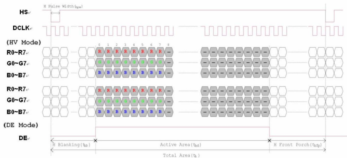
Figure 7. Horizontal input timing diagram
