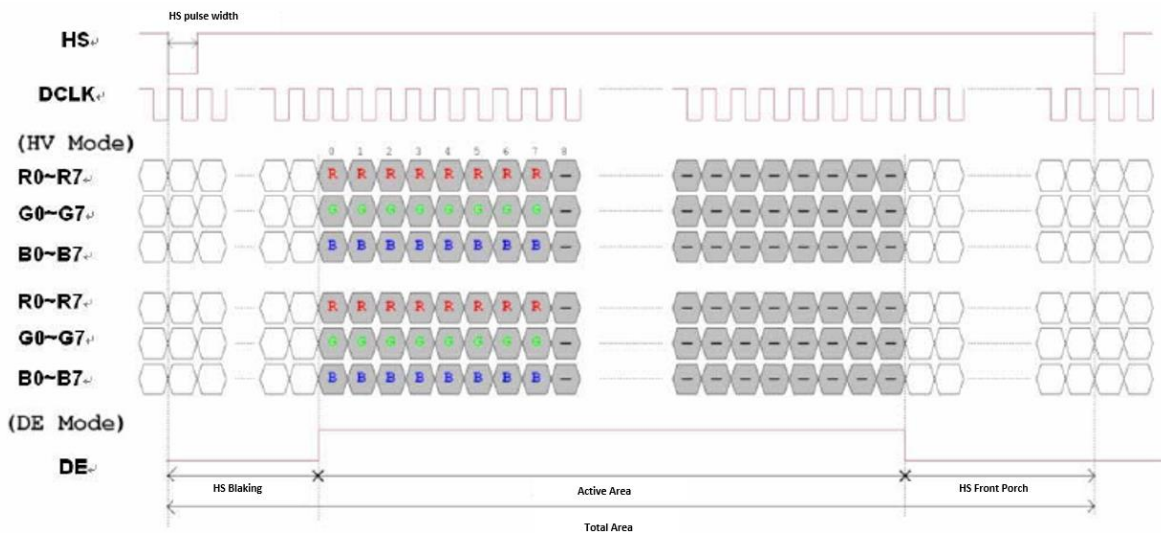
Figure 4. Horizontal input timing diagram
