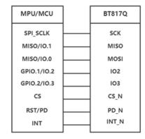
**SPI Interface** – the SPI slave interface operates up to 30MHz (It depends on EVE4 system clock frequency and needs verification in Riverdi lab).
