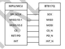
Figure 7. QSPI interface connection
