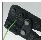
③ Grip the handles steadily until ratchet is released.
