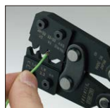
② Insert wire into barrel of contact.
