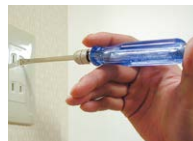
Circuit testing handle (AC80~300V/DC100~250V)
