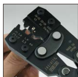
① Put a contact pin to hold.
