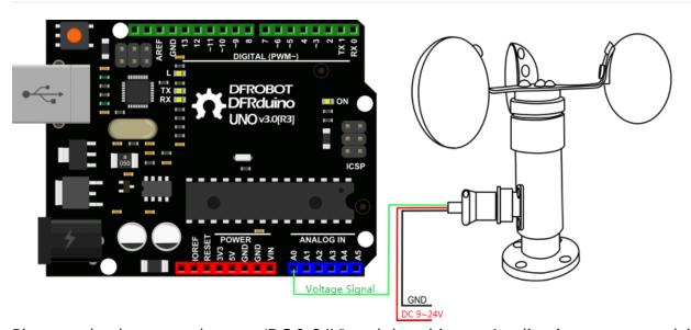
Please make the external power (DC 9-24V) and the wiring to Arudino in same ground, i.e. connect GND to arduino as well as to external power's GND. In the diagram, it was not indicated out.
