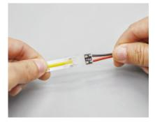
Insert one end of led strip and wire connector into both ends of the connection terminal respectively to ensure that the metal clip is on the same side as the metal solder pad of led strip
