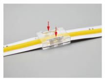
Press the metal clip down with the appropriate force using pliers to ensure that the metal clip is inserted into the appropriate position ,and connection completed.
