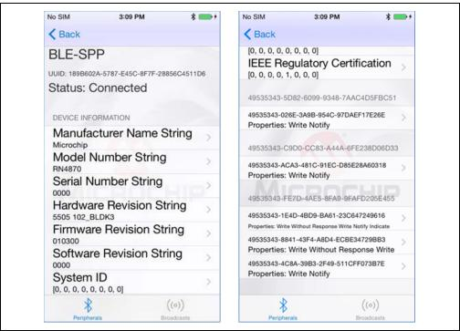
6. Click any of the listed characteristics that the SmartDiscover App discovered to look for the details of the characteristic, such as: name, UUID, access properties, and notification/indication; and also to enable notification and read and write the characteristic based on the access supported. Refer to Figure 4-3.
