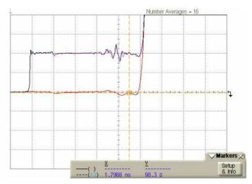
Figure 2 - TDR Measurement with 200ps risetime using Semtech Evaluation Board
