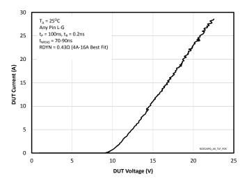
ESD Clamping (-8kV Contact per IEC 61000-4-2)
