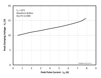
ESD Clamping (+8kV Contact per IEC 61000-4-2)
