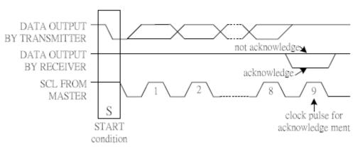
Fig .9.4 Acknowledgement on the 2-line Interface
