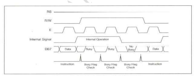
Example of 8-bit Bus Mode Timing Sequence
