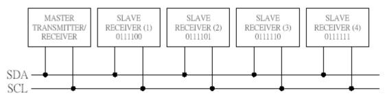
Fig .9.3 System configuration
