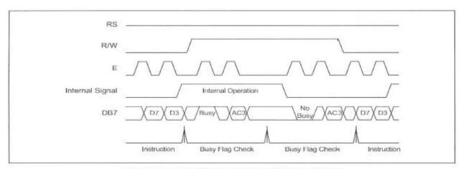
Example of 4-bit Bus Mode Timing Sequence
