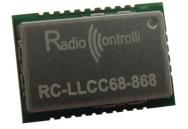
LoRa Smart Home (LLCC68) is a sub-GHz LoRa® RF Transceiver for medium range indoor and indoor to outdoor wireless applications. SPI interface. Designed for long battery life with just 4.2 mA of active receive current consumption. The LLCC68 can transmit up to +22 dBm with highly efficient integrated power amplifiers.
