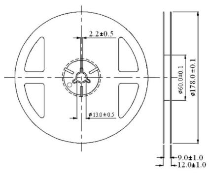
Unit: mm Tolerance:  $\pm 0.25$ mm
