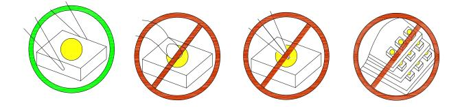
Compare to epoxy encapsulant that is hard and brittle, silicone is softer and flexible. Although its characteristic significantly reduces thermal stress, it is more susceptible to damage by external mechanical force. As a result, special handling precautions need to be observed during assembly using silicone encapsulated LED products. Failure to comply might lead to damage and premature failure of the LED.
