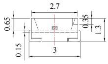
**Recommended Soldering Pad Dimensions**
