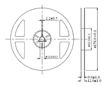
Unit: mm Tolerance:  $\pm 0.25$ mm
