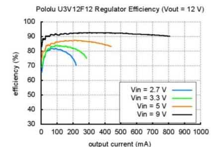
The maximum achievable output current is approximately proportional to the ratio of the input voltage to the output voltage. If the input current exceeds the switch current limit (typically somewhere between 1.4 and 2 A), the output voltage will begin to drop. Additionally, the maximum output current can depend on other factors, including the ambient temperature, air flow, and heat sinking.
