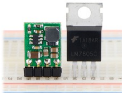
Pololu step-down voltage regulator D24VxFx next to a 7805 voltage regulator in TO-220 package.
