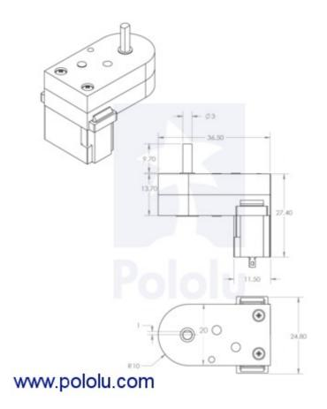
Dimensions (in mm) of the 120:1 and 180:1 mini plastic gearmotors with offset 3mm D-shaft outputs.
