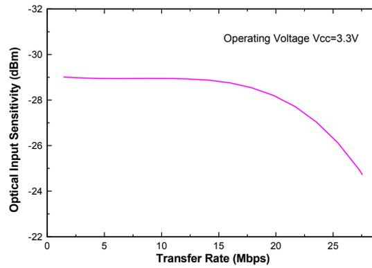
**Note:** Before using the PLR233 series device, please confirm the minimum sensitivity at different operating voltage and transmission rate.
