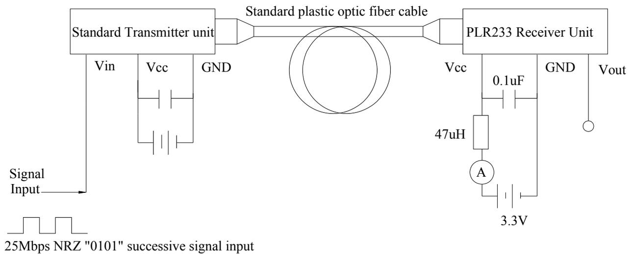
\*Fig.3 Measuring Method of Output Voltage, Pulse and Jitter
