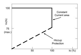
Typical LED power supply I-V curve
