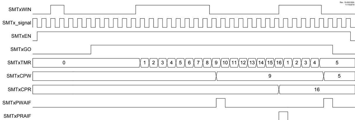
**Figure 27-22. Windowed Counter Mode, Single Acquisition Timing Diagram**
