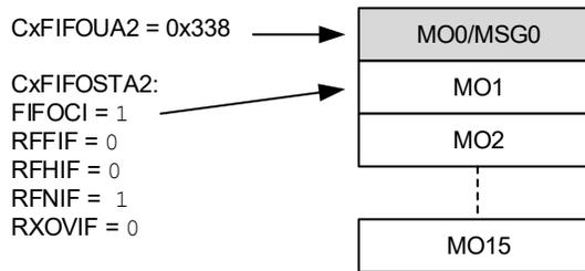
Figure 38-26 illustrates the status of FIFO 2 after MSG0 is read. The user application reads the message from RAM and sets the UINC bit (CxFIFOCON2[8]). The user address increments and points to MO1. The FIFO index is unchanged. The FIFO is empty again. All flags are cleared.
