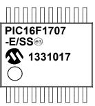
20-Lead SOIC (7.50 mm)
