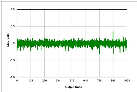
**FIGURE 38-33:** ADC, DNL,  $V_{DD} = 3.0V$ ,  $T_{AD} = 1\ \mu\text{S}$ ,  $25^\circ\text{C}$ .
