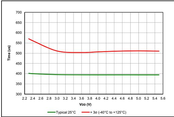
**FIGURE 38-31:** Wake From Sleep,  $V_{REGPM} = 1$ ,  $LFINTOSC$ , PIC16F18857/77 Only.
