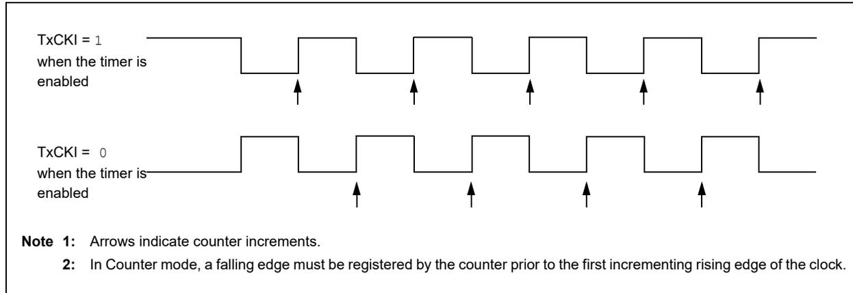
**FIGURE 28-3: TIMER1 GATE ENABLE MODE**
