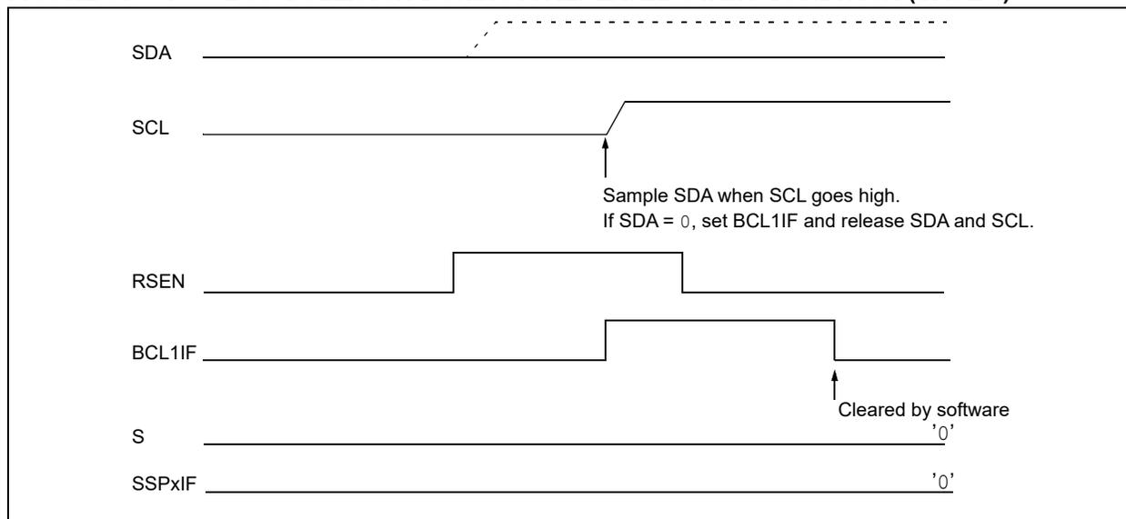
**FIGURE 31-37: BUS COLLISION DURING REPEATED START CONDITION (CASE 2)**
