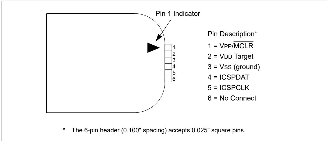
**FIGURE 35-3: TYPICAL CONNECTION FOR ICSP™ PROGRAMMING**
