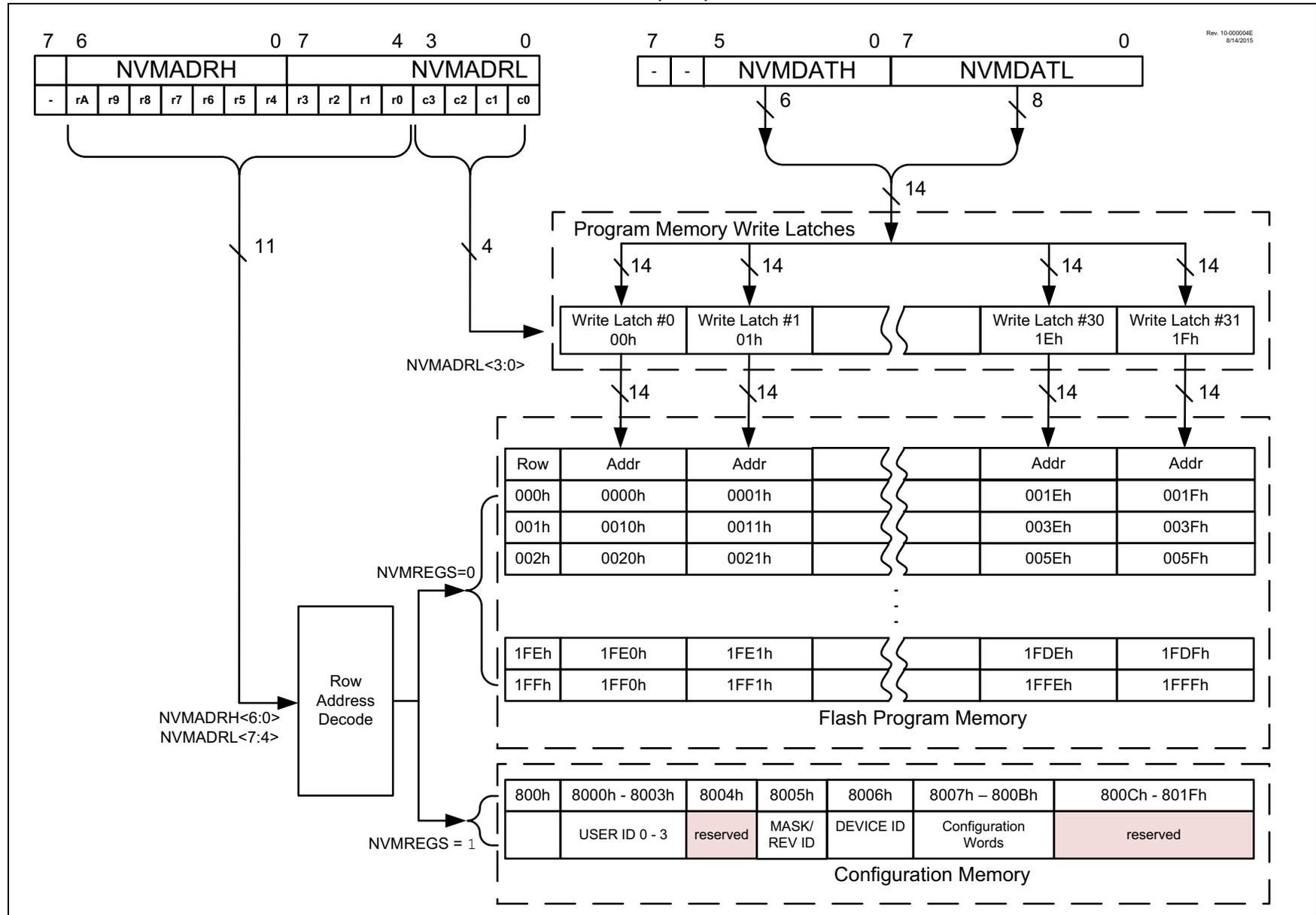
**FIGURE 10-5: PROGRAM FLASH MEMORY (PFM) WRITE FLOWCHART**
