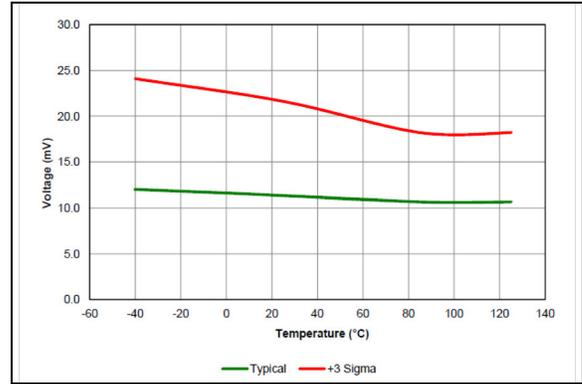
**FIGURE 38-16:** Brown-Out Reset Hysteresis, Trip Point (BORV = 1x).
