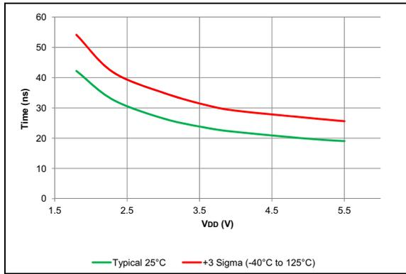
**FIGURE 38-85:** Fall Time, Slew Rate Control Enabled.
