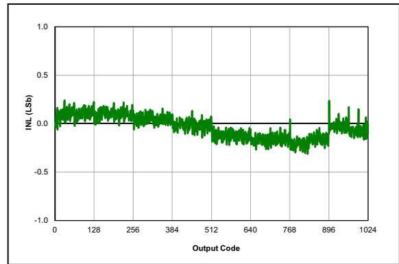
**FIGURE 38-35:** ADC, INL,  $V_{DD} = 3.0V$ ,  $T_{AD} = 1\ \mu\text{S}$ ,  $25^\circ\text{C}$ .
