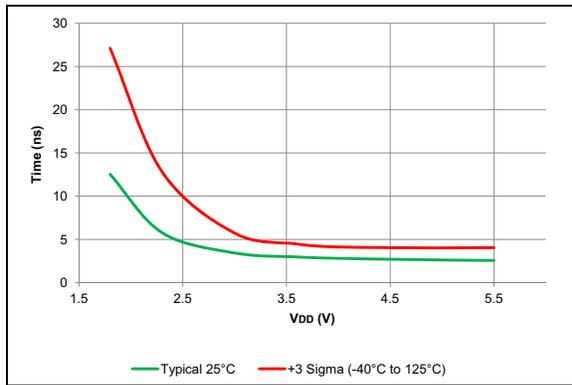
**FIGURE 38-86:** Rise Time, Slew Rate Control Disabled.
