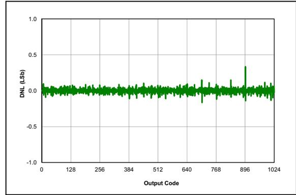
**FIGURE 38-34:** ADC, DNL,  $V_{DD} = 3.0V$ ,  $T_{AD} = 4\ \mu\text{S}$ ,  $25^\circ\text{C}$ .
