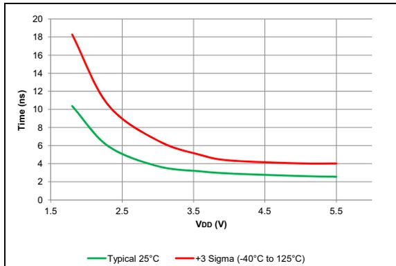
**FIGURE 38-87:** Fall Time, Slew Rate Control Disabled.
