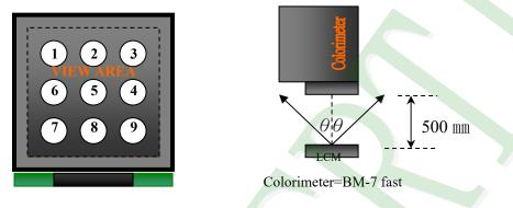
To be measured at the center area of panel with a viewing cone of 1° by Topcon luminance meter BM-7, after 10 minutes operation (module)
