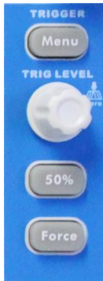
Figure 0-12 Trigger Control Zone
