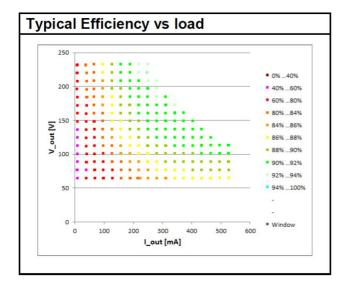
OTI DALI 60/220-240/550 D LT2 L Typical Efficiency vs. Load (230 V / 50 Hz)
