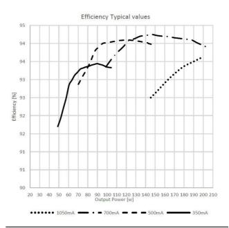
OT DX 200 G2 Typical Efficiency vs. Load (230 V 50 Hz)
