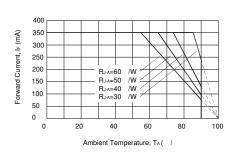
Note: Don't drive at rated current more than 5s without heat sink for Xeon 1 emitter series.
