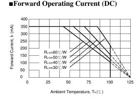
Note: Don't drive at rated current more than 5s without heat sink for Xeon 1 emitter series.
